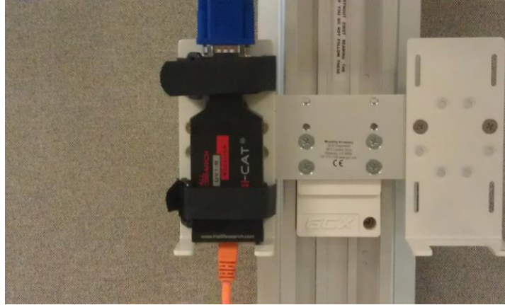
Figure 18 – UV1-R Video Receiver Mounting
